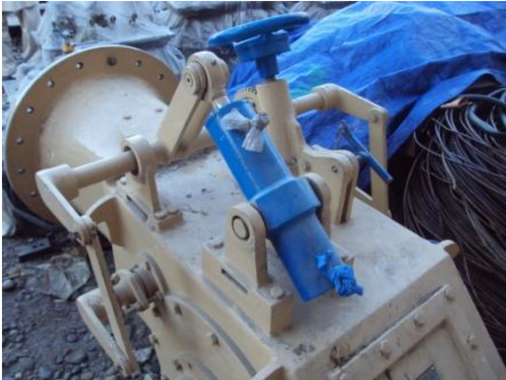
Fig. 4. Pakistani cross flow Turbine by SK Company for 200 kW system in Kodikhil (pending)
