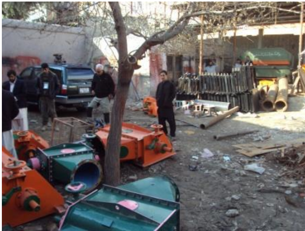
Fig. 5. Shenwar Kharadi Workshop / Cross flow turbine manufacturer
